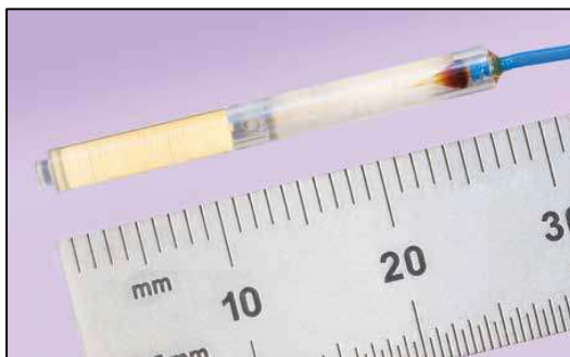
Figure 3: Passive sensor for multi-axis, fiber-based position measurement.
