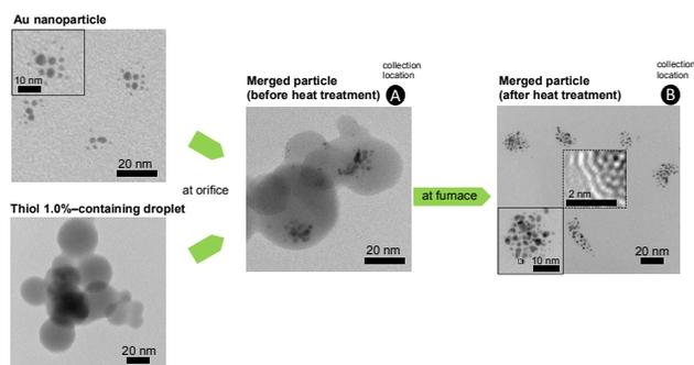
Figure 4: TEM images of spark generated Au and collision atomized hexanethiol/EtOH (left), and merged (center, before passing through the tube furnace; right, after passing through the tube furnace) particles.
