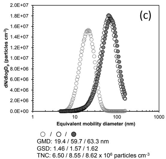
Figure 3: Size distributions of the spark generated Au, collision atomized hexanethiol/EtOH, and merged particles. The fabrication was applied using (a) 0.1% (v/v), (b) 0.5% (v/v), and (c) 1.0% (v/v) thiol concentrations (in EtOH). The spark generated Au, hexanethiol/EtOH, and merged particles are gray (unfilled), black (unfilled), and black (gray filled) circles, respectively.
