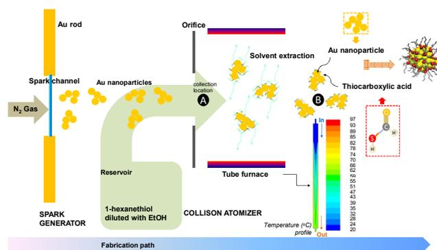
Figure 1: Aerosol based fabrication of thiol-capped Au nanoparticles.
