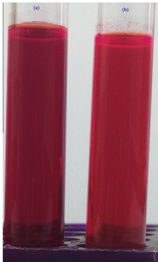
Fig. 2. The real pictures of the filtered solutions of the TDCV-TPA for 2 mM dissolved in (a) DCM and (b) chloroform solvent.
