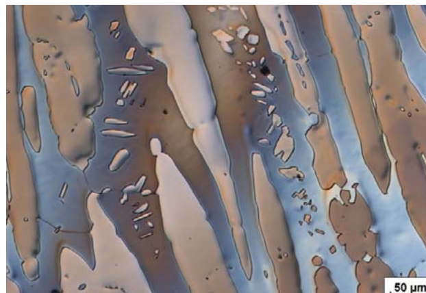
Fig. 11: Corrosion-resistant austenitic-ferritic steel (duplex) following electrolytic etching in 20 % sodium hydroxide solution. The austenite grains (light brown) are embedded in the bluish-brown ferritic matrix.
