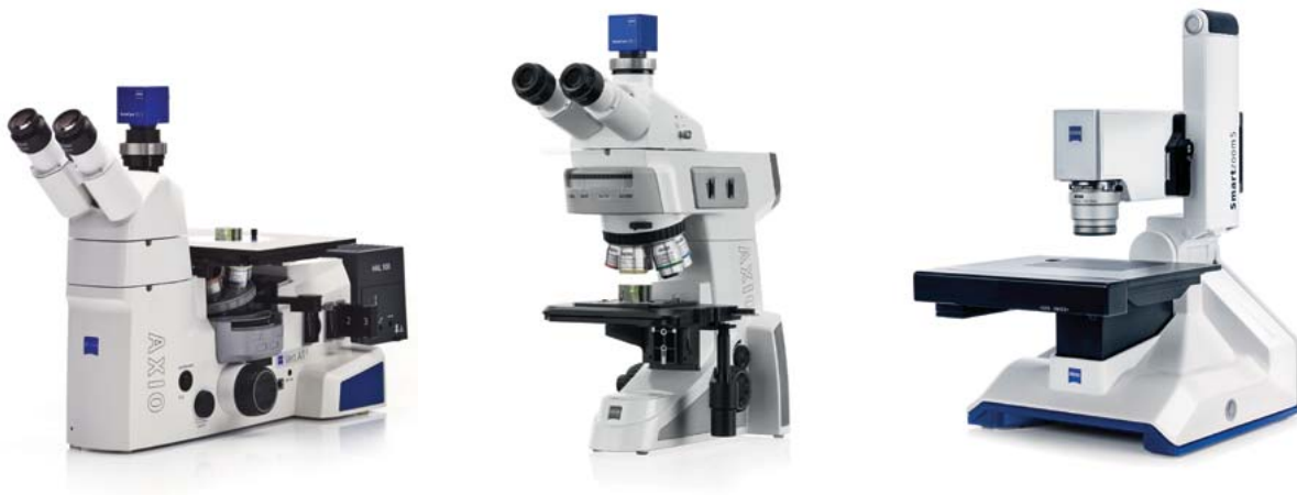
Fig. 20: Versions of light microscopes for structural analyses. In addition to inverted and upright material microscopes (such as the A ZEISS Axiovert.A1 MAT and ZEISS AxioLab.A1 MAT), digital microscopes such as the ZEISS Smartzoom 5 are increasingly becoming an alternative.
