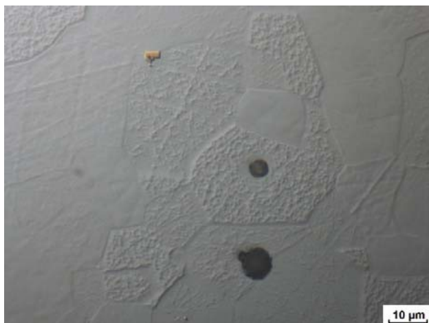
Fig. 9: Ferritic steel with titanium carbide and oxide inclusions following mechanical preparation to 1 μm diamond. Fine traces of deformations can still be observed in the differential interference contrast image. The sample has not been etched.
