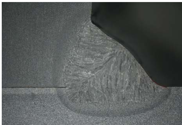
Fig. 8: Welding seam ground on two levels of SiC film, followed by macro etching with 5 % aqueous nitric acid.
