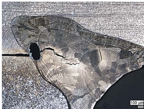
Fig. 12: Laser welding seam on high-alloy steels with fissures and pores following electrolytic etching. These are also visible in the unetched condition, but the intercrystalline course of the fissures can only be evaluated after etching has been completed.
