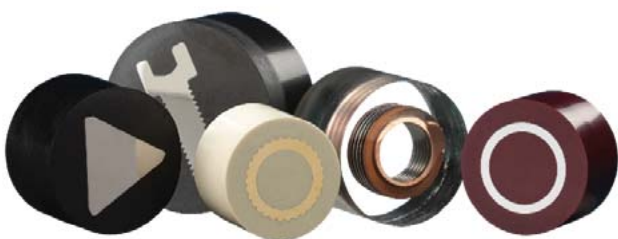
Fig. 7: Variety of embedded samples of varying shapes. Performing embedding with various synthetic resins ensures a good preparation process outcome and makes this procedure efficient.
