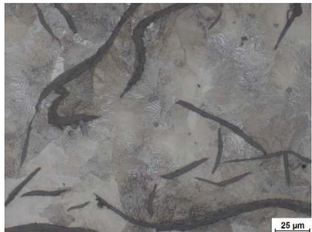
Fig. 2: Pearlitic cast iron with lamellar graphite, etched with nital. The carbon is primarily present as graphite in a lamellar form, which results in reduced strength. The pearlitic matrix itself exhibits a sufficiently high degree of hardness.
