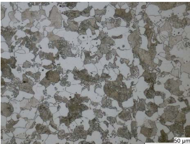
Fig. 5: Ferritic-pearlitic steel with approx. 0.2 % C, etched with nital. The carbon is primarily present as a cementite lamella in a harder proportion of pearlite adjacent to the ferritic grains. This causes the cementite to appear streaky. The pearlitic grain reflects less light than the ferritic grain and thus appears darker. A matrix of this type has a higher degree of hardness than the steel in image 4, but a lower resilience.
