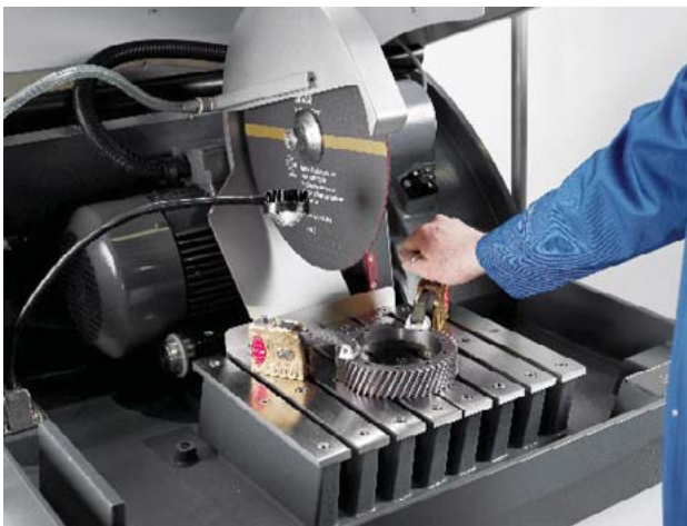
Fig. 6: Wet abrasive cutting machine with clamped gear wheel for taking a sample of a section of a gear tooth. This section, which is typically induction- or case-hardened, will be examined with respect to its structure and hardness and thus needs to be separated from the component.
