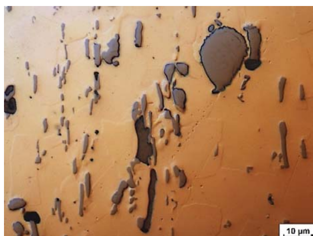
Fig. 15: Copper alloy like that in Fig. 14. Due to their ablation behavior, the phases of varying hardnesses have varying heights, which are only visible in DIC microscopy. This enables a qualitative distinction between their hardnesses. At the same time, the grain structure can already be made visible in the unetched condition.
