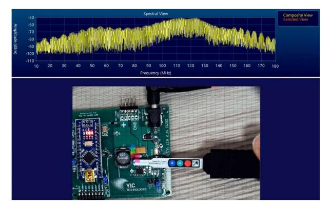
Live tracking provides a faster, easier, and more reliable method to get these results. Using an overhead webcam and probe markers, the EMViewer software will detect the type of probe and point of measurement automatically, allowing design engineers to see results quickly with minimal setup time.
