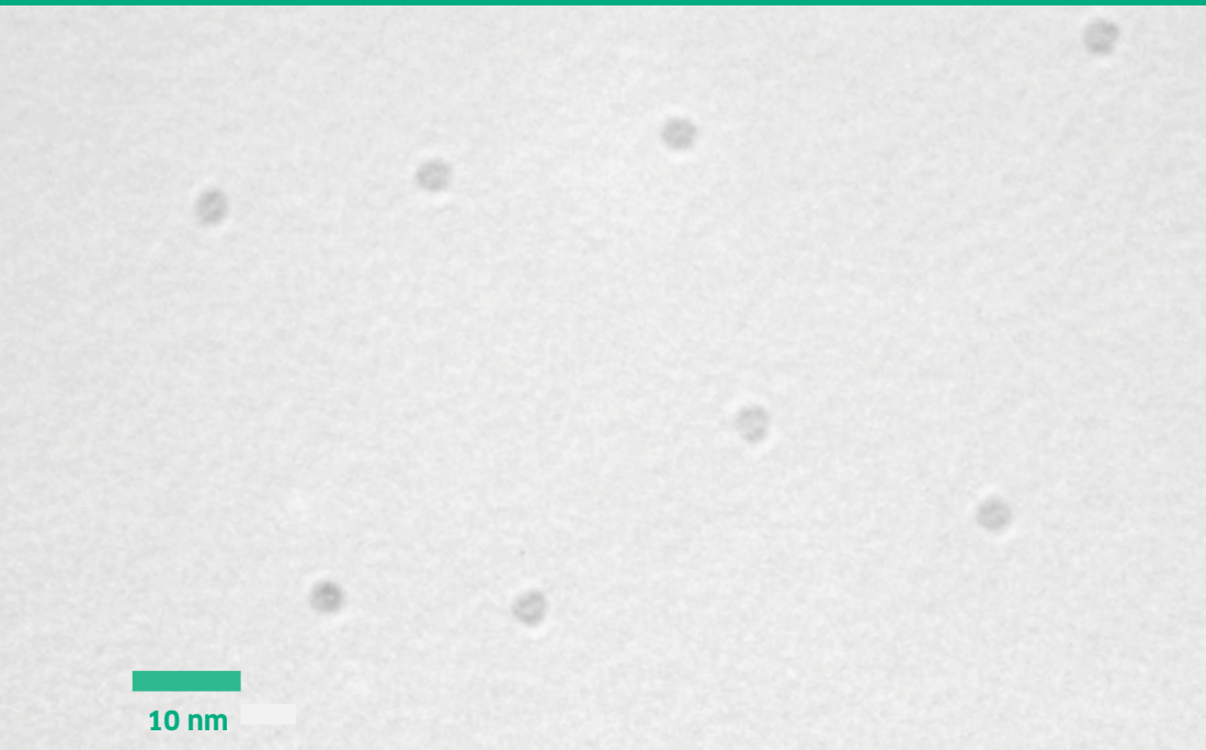
3 nm Au nanoparticles on an in-situ TEM chip prepared with the VSP-G1 and VSP-S1
