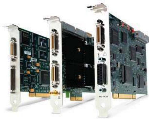
Figure 5. National Instruments frame grabber cards for desktop computers
