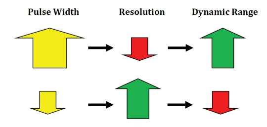
Measurements with a short Pulse Width and a Long Pulse Width
