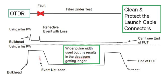
Here you can see that with a 5ns pulse width the fault can be easily measured but the end of the fiber can't be seen. If a wider pulse width is used (1us) the fault can no longer be
