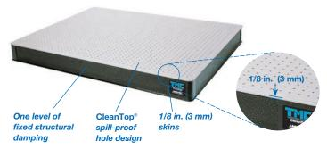
TMC's 78 and 77 Series CleanTop® Breadboards provide the ultimate in rigidity and damping for smaller tops. Available in both 2 and 4 in. thicknesses (50, 100 mm), these tops include the same proprietary CleanTop spill-proof hole technology and small cell, high-density steel honeycomb core as our largest tops. These tops can be readily designed to meet custom requirements including custom mounting hole patterns, through-holes, special shapes and custom materials.
