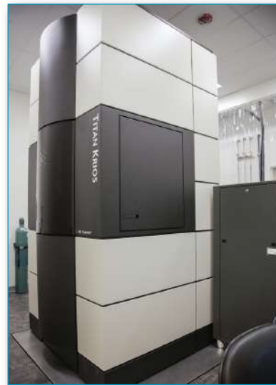
Thermo Fisher Titan Krios Cryo Transmission Electron Microscope supported by a STACIS platform at Oregon Health Sciences University.
