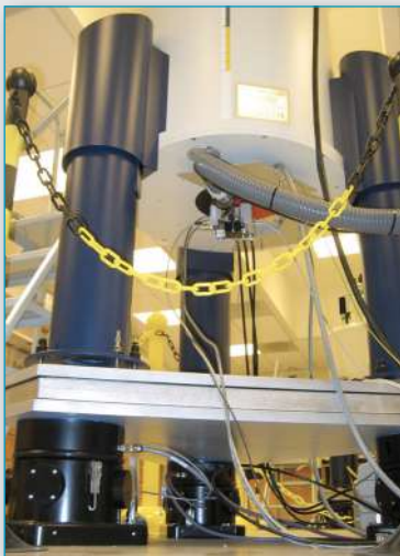
A STACIS ® System, incorporating a non-ferromagnetic, highly damped, aluminum platform, provides a second stage of vibration isolation for a Bruker BioSpin 600 MHz NMR Spectrometer. Photo courtesy of Bruker BioSpin and Memorial Sloan Kettering Cancer Center.
