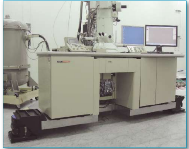
STACIS® Floor Platform supporting a JEOL JEM-2100F Transmission Electron Microscope (TEM).
