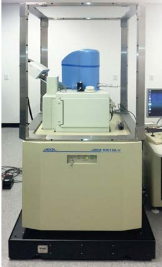
Column-mounted Helmholtz Coils are readily adapted to SEM columns but impractical for TEMs.
