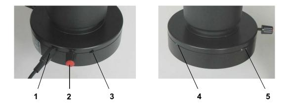
Insert the barrel connector (1) of the power supply (F) into the DC socket provided on the ringlight (A). The plug connection of the power supply is interchangeable for the EU, UK, US and AU. The plug connection needs to be connected to the mains supply (100-240 V AC, 50-60 Hz).
