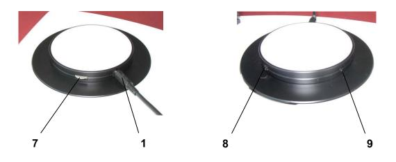
Insert the barrel connector (1) of the power supply (F) into the DC socket provided on the Transmitted Light Stage (B). The plug connection of the power supply is interchangeable for the EU, UK, US and AU. The plug connection needs to be connected to the mains supply (100-240 V AC, 50-60 Hz).
