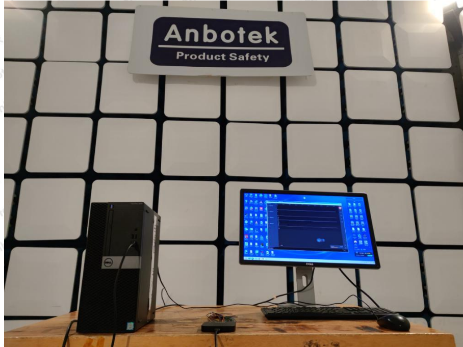
Photo of RF Field Strength susceptibility Test
