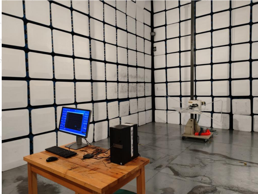
Photo of Radiated Emission Test
