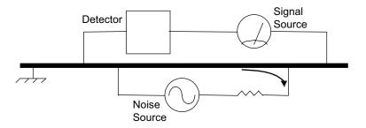
In this illustration, the detector is measuring the signal relative to a ground far from the rest of the experiment. The detector senses the signal plus the voltage due to the noise source's ground return passing through the finite resistance of the ground between the experiment and the detector. The detector and the experiment are grounded at different places which, in this case, are at different potentials.
