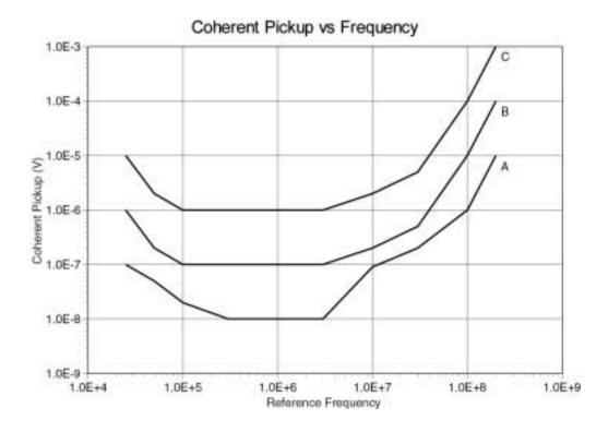
The level of coherent pickup (three curves above) is dependent on the RF input gain. The choice of Wide (RF) reserve and Sensitivity determines the RF gain and thus, the level of coherent pickup. The following table shows which curve to use.
