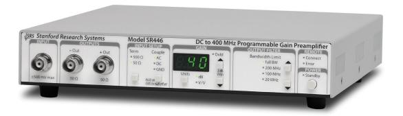
The SR446 is a single-channel, 400MHz bandwidth voltage preamplifier with 21 programmable gains from 1 to 100 (+0 dB to +40 dB with 2 dB steps). It also includes four programmable low-pass filters, with settings of full bandwidth, 200 MHz, 100 MHz and 20 MHz. There are two output channels which offer complimentary outputs (inverting and non-inverting) that can be used separately, or together as a differential output.
