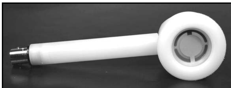
Figure 31. The Crystal Holder with a 1 inch sensor crystal mounted.
