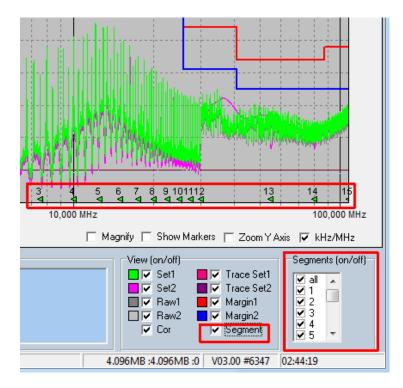
As Quasi-Peak measurements take much time, an alternative measurement method is available. A peak-scan would only look at frequencies, which come close to the limit or which exceed the limit in Peak or Average mode.
