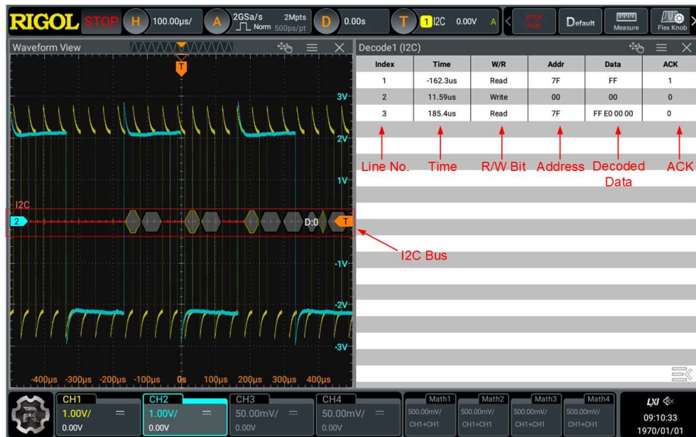
Figure 15.10 I2C Decoding Event Table
