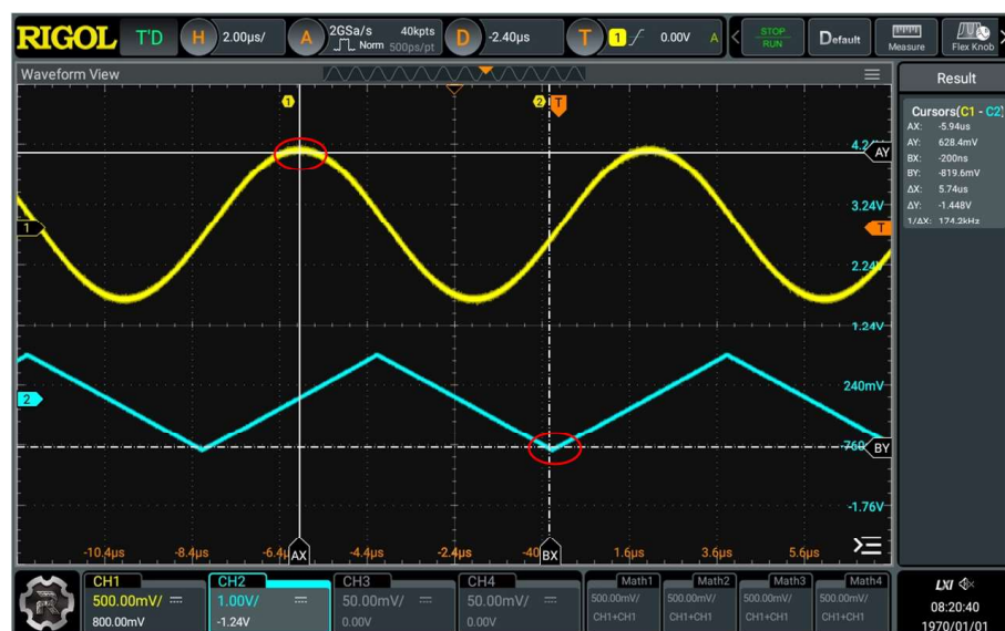
Figure 10.13 Track Measurement (after Horizontal Expansion)
