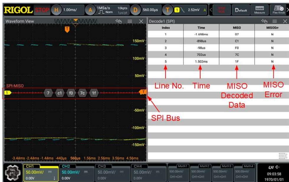
Figure 15.13 SPI Decoding Event Table
