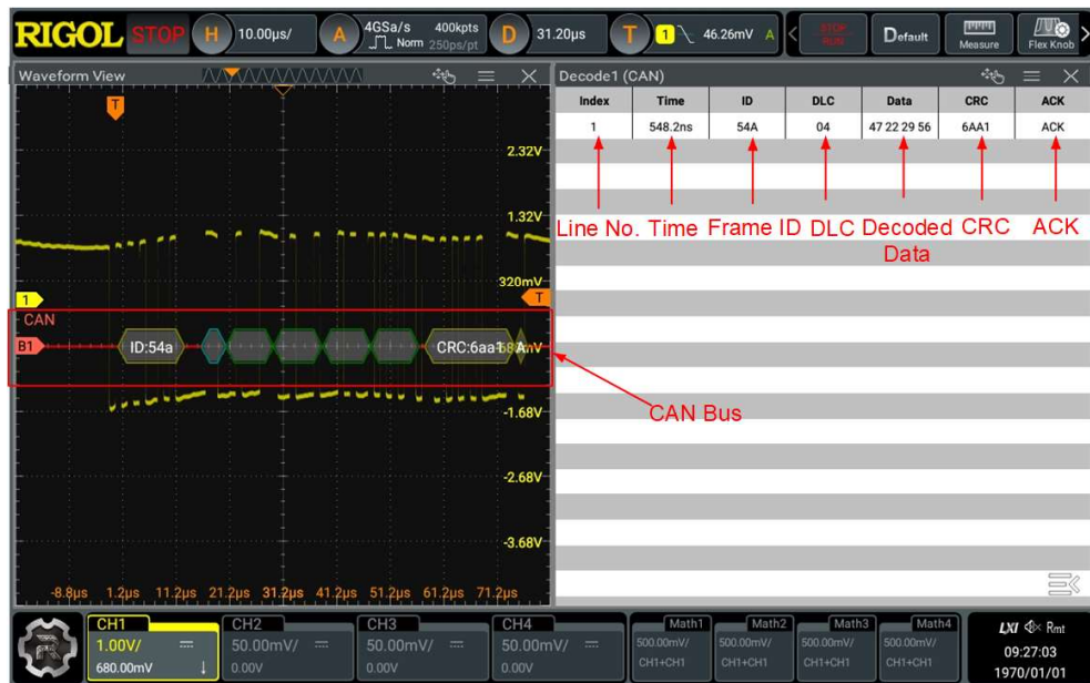
Figure 15.18 CAN Decoding Event Table
