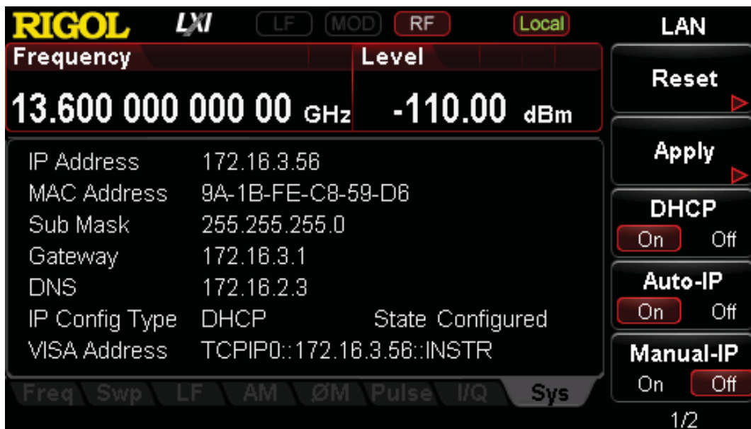
Figure 2-3 To Set the LAN Parameters
