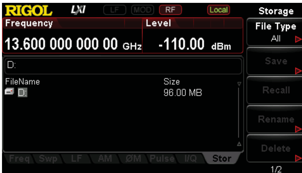
Figure 2-1 store and recall interface
