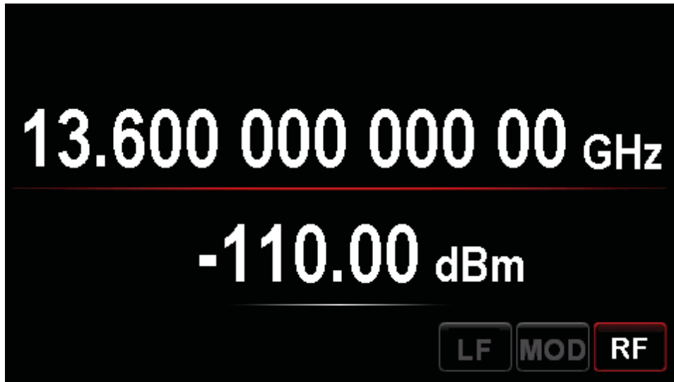
Figure 1-10 User Interface (Parameter Zoom-in Mode)
