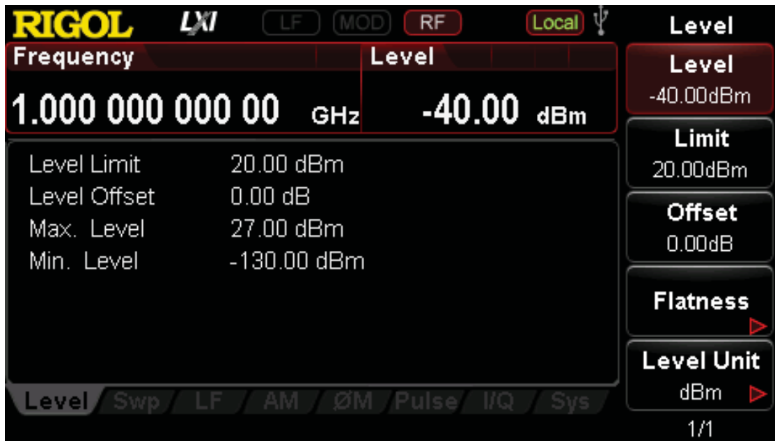
Figure 4-1 Parameter Setting Interface of RF Signal Output
