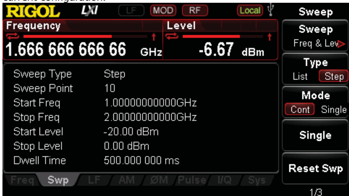
Figure 10 Parameter Setting Interface of RF Sweep Signal Output
