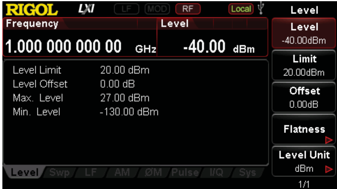
Figure 9 Parameter Setting Interface of RF Signal Output
