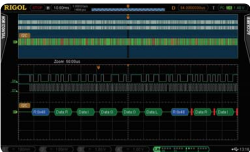
Serial bus triggering and decoding on digital channels
