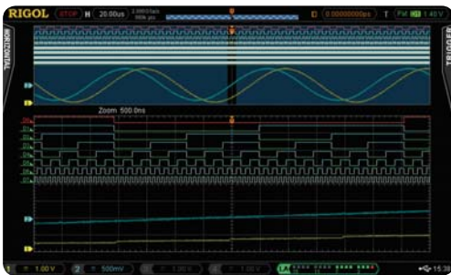
Serial bus triggering and decoding on digital channels
