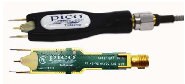
Fig. 7. Practical realisation of low-cost precision passive probe.
