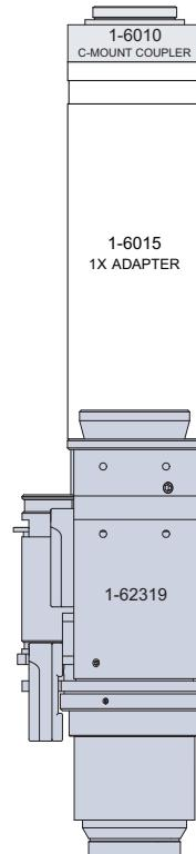
Zoom 6000 configuration with motorization and right angle adapter
