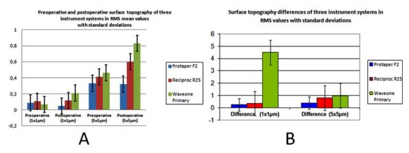
Fig. 2. A: Preoperative and postoperative surface topography and (B) surface topography change scores of three instrument systems: mean RMS scores with SDs (P < 0.1). [Color figure can be viewed in the online issue, which is available at wileyonlinelibrary.com.]
