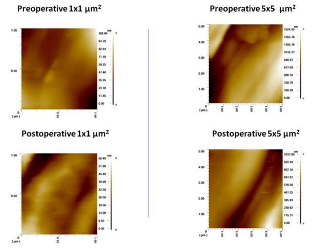
Fig. 1. Three-dimensional AFM images of a representative point on a WaveOne Primary file obtained from preoperative and postoperative  $1\times1$  and  $5\times5\,\mu\text{m}^2\text{scanning}$  processes. [Color figure can be viewed in the online issue, which is available at wileyonlinelibrary.com.]
