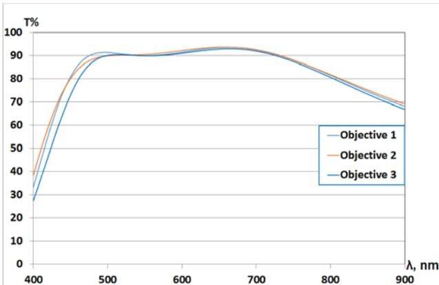
Fig.3. Actual spectral transmittance of individual short-throw mini-objectives.
