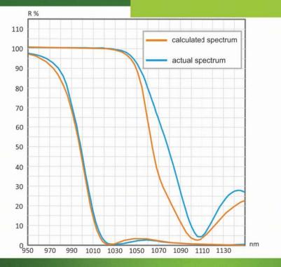
Thin film polarizer optimized for maximum efficiency at 1030 nm / 56 deg AOI.
