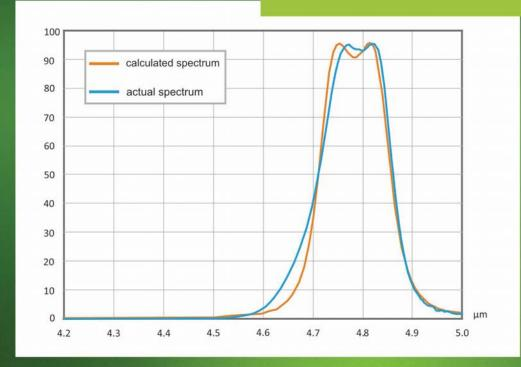
IR band-pass filter with 19 layers optimized at 4,78 μm. The Si/SiO layer stack is coated on sapphire substrate.
