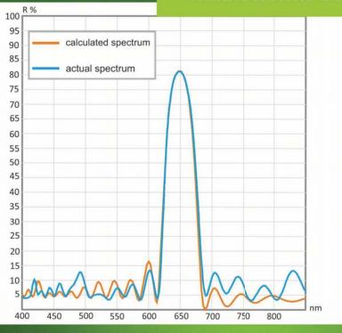
Target specifications: Rmax ≥ 80% @ 650 nm FWHM ≤ 55 nm
