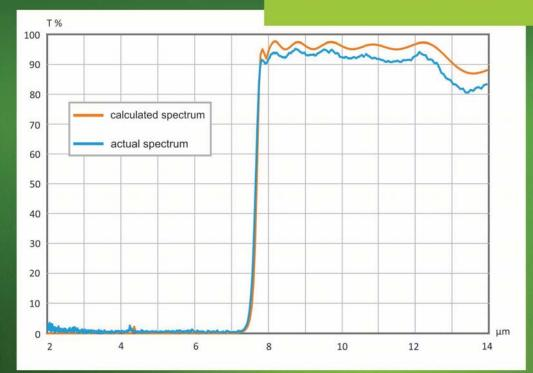
IR longpass filter produced on Ge substrate, with broadband (8-14  $\mu$ m) AR coating on the back side.
