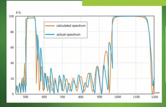
Multilayer interference mirror at two wavelengths – 532 nm and 1064 nm. The thin film stack is designed for operation at 0 deg AOI.
