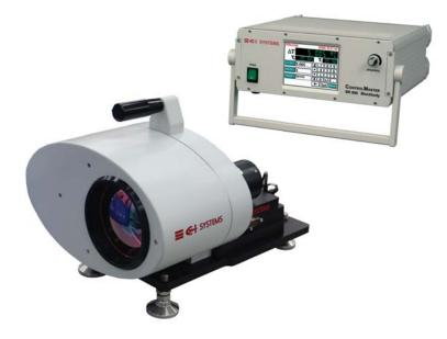
The wide field of view IR test collimator, is used to test thermal imagers in their wide field of view mode of operation. Typical applications include navigational FLIR's and commercial imagers. CI's unique compact WFOV is an IR collimator combined with an accurate IR source (CI's SR 800-2D) and a target wheel. The WFOV provides the means to perform IR testing such as; MTF, NETD, MRTD etc.
