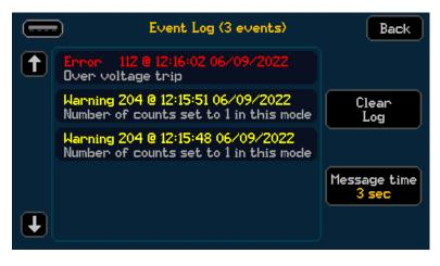
Selecting the Event Log symbol on the status bar will open the event log menu, this menu can also be accessed through the System menu: CNFG > [System] Event Log. Within the Event log menu, the events are colour coded and include a Warning or Error number alongside the time and date of when the error occurred.
