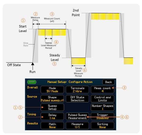
The time it takes to complete one single sweep can be calculated by = (Number of Points x ((Settling Delay x 2) + (Sweep Measurement Period X Measurement Count) + (Pulse Steady Level Measurement Period))).
