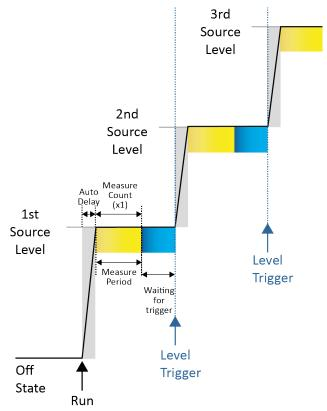
The input trigger can also be used to repeat shape waveforms, in order to source the next waveform shape.
