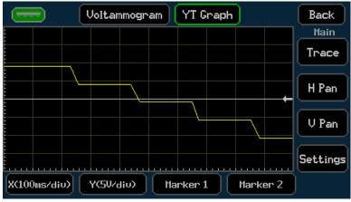
Point: Show each measured point on the graph as a single pixel.
