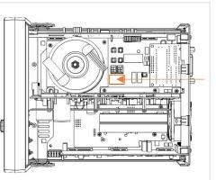
(2) Remove 2x screws from the rear panel.
