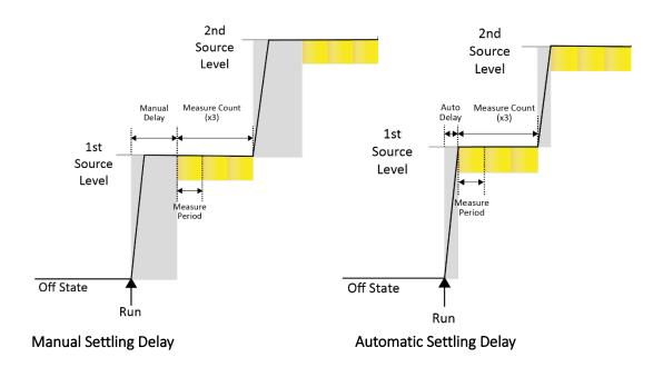
The actual source settling time is dependent upon many factors including mode, slew rate, load, magnitude of change, polarity change etc. As such, careful consideration needs to be made when deciding upon the delay. See *'Specification'* for more details on source settling times.
