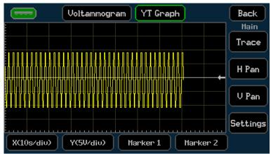
To change the scale, select the X (xxx/div) or Y (xxx/div) button located at the bottom of the graph. The X and Y axis will remain in the automatically selected ranges until modified. A green outline will appear to show the range can now be changed, use the encoder to change the range, the scale will then be adjusted using units per division.
