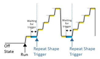
The global input trigger event can be provided by remote command using the command SYST[em]:TRIG[ger] or from pin 8 on the DIO port.
