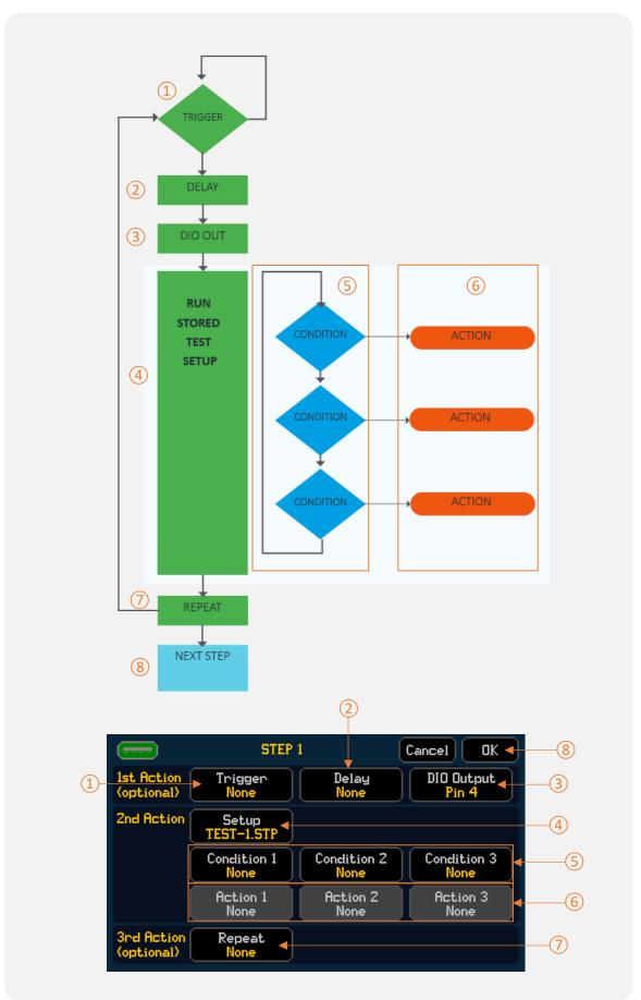
Once a setup has been added, actions and conditions can be added to the sequence step.
