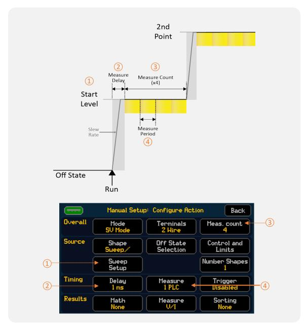
The time it takes to complete one single sweep can be calculated by = (Number of Points x (Settling Delay + (Measurement Period x Measurement Count))).
