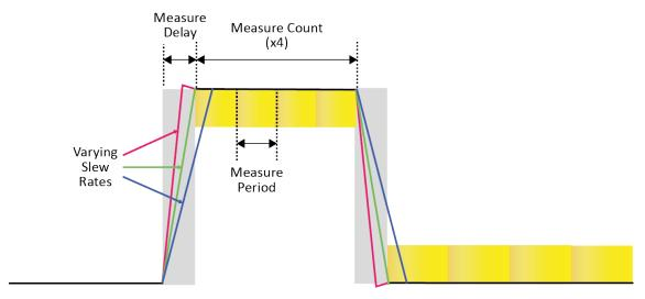
It is important to note that this is a maximum setting and does not precisely define the rate of change, as the source output transition rate can be affected by other factors including output level, load level, voltage, and current and load reactance.
