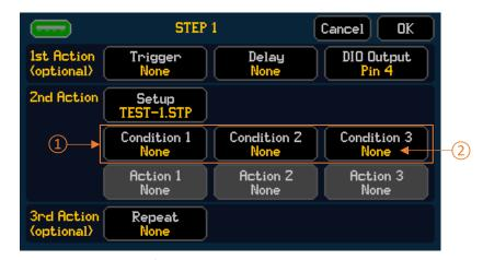
The conditions for the  $2^{nd}$  Action (1) are performed/checked in order. For example, if only Condition 3 (3) is set then two cycles (~150ms) will be needed prior checking that condition.
