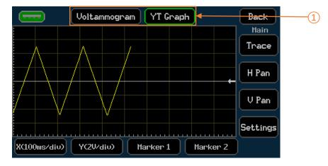
**Voltammogram** (I/V Scatter): A plot of voltage against current. This graph type is ideal for I/V curve tracing.
