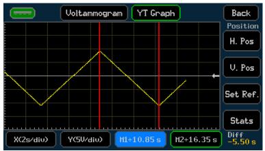
A reference point based on the selected marker (used in the math function) can be set directly from the graph using the **Set Ref** button. See '*Math*' for more details.
