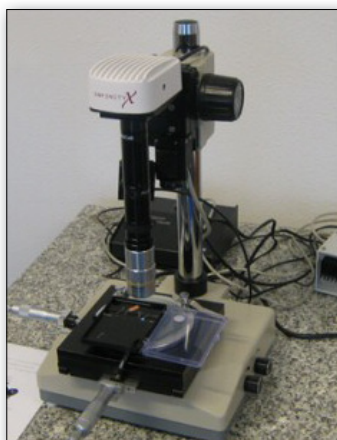
Inspection of Atomic Force Microscope (AFM) probes using Navitar Ultra Precise Eye. Image courtesy of DeltaPix.
